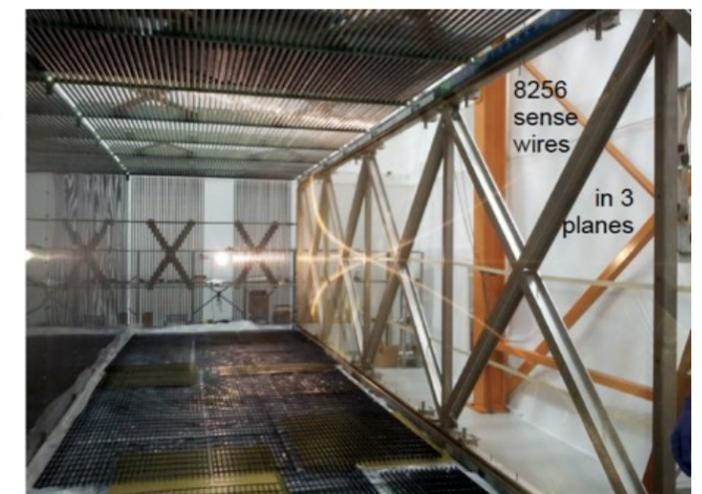
The wire cage that surrounds the detection volume is about 3m x 3m x 10m. This gets put into a huge tank (the cryostat) which holds 170 tons of liquid argon. (Continued on page 2)
